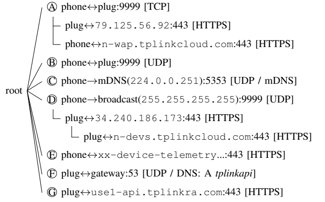
Fig. 5: Event signature tree for the TP-Link HS110’s toggle event. Bidirectional flows are represented by a double-headed arrow, whilst a single-headed arrow is used for unidirectional flows. When indicated, the port is associated with its host.
