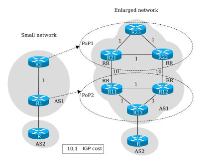
Fig. 4. Enlarging a network
