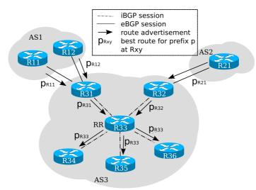
Fig. 1. Example of route diversity loss. Location of eBGP peerings: R31 selects either  $p_{R11}$  or  $p_{R12}$  as best route. R31 only propagates this route in iBGP. eBGP attributes of the routes: If R32 assigns a high Loc\_pref to  $p_{R21}$ , neither  $p_{R11}$  nor  $p_{R12}$  will be propagated in iBGP. iBGP propagation graph: R33 selects either  $p_{R31}$  or  $p_{R32}$  as best route. R33 only sends this route to R34, R35 and R36.
