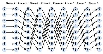
Fig. 2: The Linear-shift scheduling with 8 servers.
