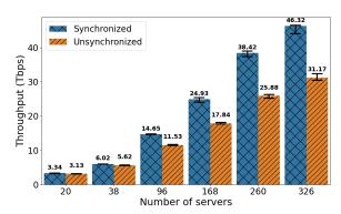
Fig. 6: Scalability of the synchronized and non-synchronized all-to-all applications. The error bars represent the minimum, mean and maximum values.
