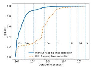
Fig. 3: Cumulative distribution of failure duration. The blue line represents the cumulative distribution of failure duration without the flapping links correction. The orange dotted line represents the cumulative distribution of failure duration with the flapping links correction. Flapping links correction is applied by counting failures of a flapping link as one long failure rather than several small failures spaced over a short period of time.
