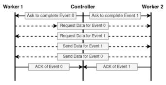
Fig. 5: Description of the MPI all-to-all application without synchronization.
