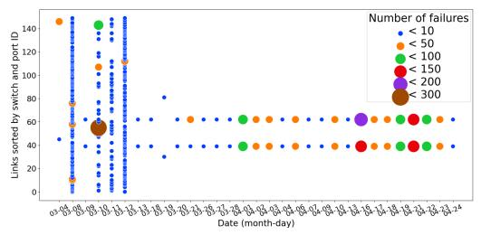
Fig. 4: Distribution of network link failures over a two-month period. The x-axis represents the days in March and April 2024 when failures occurred. The y-axis represents the IDs of the links that failed during this period. The link IDs are assigned based on the switch IDs and the port IDs which are sorted in ascending order.
